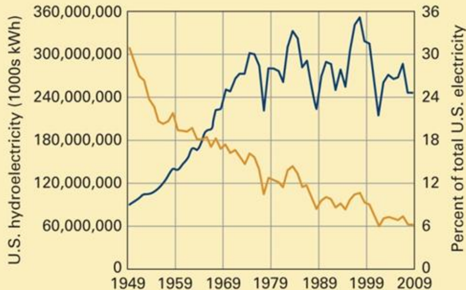
Figure 11.21: Fraction of electricity from hydroelectric generation in the United States as a function of year (yellow line), along with the total hydroelectric generation (blue line).
